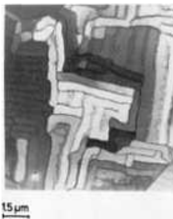
FIG. 20 LABYRINTH/CELL STRUCTURE WITH MARKED MISORIENTATION. \Delta\epsilon_{pL}/2 = 2 \times 10^{-3} , N \approx 10^4 . SOURCE: REF 101
