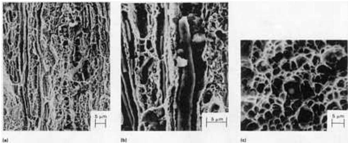
Fig. 14 Scanning electron micrographs of AISI 4130 steel. (a) and (b) Fractures of resulfurized steel that had been quenched and tempered to 1400 MPa. (c) Low-sulfur AISI 4130 steel that had been spheroidized to 600 MPa. In all three photographs, particles can be found in the dimples. Source: Metals Handbook , 9th ed., Vol 8
