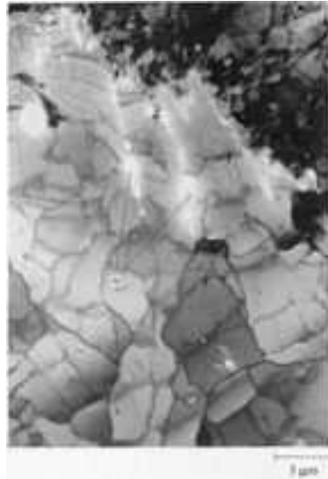
FIG. 13 SURFACE RELIEF MICROCRACKS AND DISLOCATION STRUCTURE IN SURFACE LAYER. SECTION PERPENDICULAR TO THE SPECIMEN SURFACE AND THE PRIMARY SLIP PLANE IN COPPER SINGLE CRYSTAL. D, ELECTRODEPOSITED LAYER; S, SPECIMEN; M, MICROCRACKS
