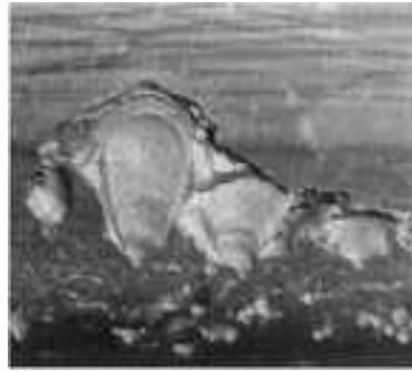
FIG. 4 FRACTOGRAPH SHOWING THE ADVANCED STAGES OF MACROPITTING FATIGUE FOR A HELICAL PINION TOOTH. COURTESY OF GEARTECH
