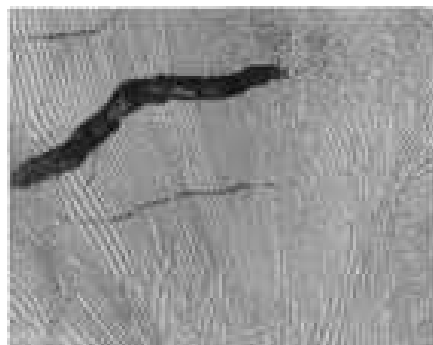
Fig. 13 Optical photograph of polished surface of a highly strained sample of experimental 0.65% C wheel steel. Initial fractures of iron carbide lamella are indicated by the arrow. The fractured lamella result in voids that link up to form a continuous fracture. Source: Ref 19
