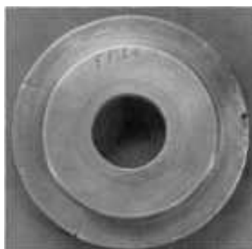
FIG. 3 DISK SPECIMEN, SHOWING RADIAL CRACKS LARGER THAN 6.35 MM, USED BY SIMOVICH (REF 34) IN THERMAL FATIGUE STUDIES ON STEELS. THE DARK SPOT AT THE RIGHT IS USED FOR TEMPERATURE SENSING.
