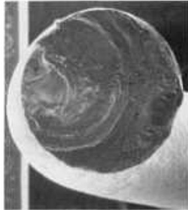
FIG. 8 SEM PHOTOMICROGRAPH SHOWING THE FRACTURE SURFACE OF A SHOT-PEENED 302 STAINLESS STEEL SPRING THAT HAD FATIGUE INITIATION AT AN INCLUSION THAT WAS 300 \mu\text{m} BELOW THE WIRE SURFACE. 21 \times
