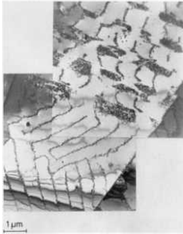
FIG. 19 DIFFERENT DISLOCATION ARRANGEMENTS WITHIN A SINGLE GRAIN OF COPPER. \Delta\epsilon_{pL}/2 = 5 \times 10^{-4} , N \approx 10^5 . SOURCE: REF 101
