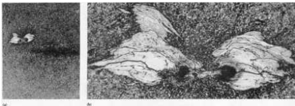
FIG. 3 MICROGRAPH SHOWING A BUTTERFLY ON A PLANE PERPENDICULAR TO THE ROLLING DIRECTION WITHIN A MARTENSITE/AUSTENITE MATRIX. (A) A SUBSURFACE FATIGUE CRACK IS VISIBLE TO THE RIGHT OF THE BUTTERFLY. 100 \times . (B) 750 \times . ETCHED IN NITAL
