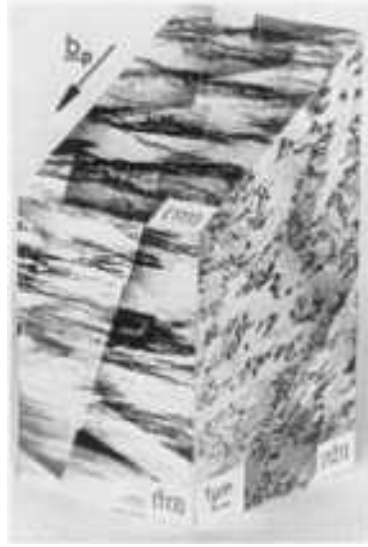
FIG. 13 THREE-DIMENSIONAL IMAGE OF THE SATURATION DISLOCATION ARRANGEMENT OF MONOCRYSTALLINE COPPER AT \gamma_{AP} = 2.6 \times 10^{-5} (REGION A). SOURCE: REF 43
