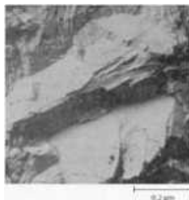
FIG. 40 CRYSTALLOGRAPHIC FACETS INDICATIVE OF SLIP-BAND CRACKING IN FE-18CR-3NI-13MN-0.37N
