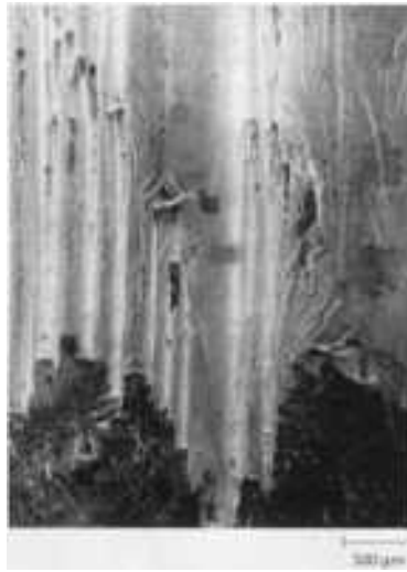
FIG. 8 CRYSTALLOGRAPHIC CRACK MORPHOLOGY FROM A CT SPECIMEN OF CMSX-2 TESTED AT ROOM TEMPERATURE WITH A SECONDARY ORIENTATION OF [110] . SOURCE: REF 103
