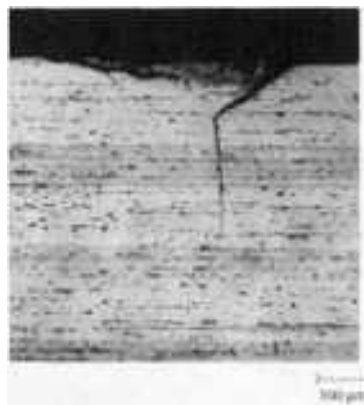
FIG. 4 EXAMPLE OF FRETTING FATIGUE CRACK VIEWED IN CROSS SECTION. COURTESY OF R.B. WATERHOUSE, UNIVERSITY OF NOTTINGHAM
