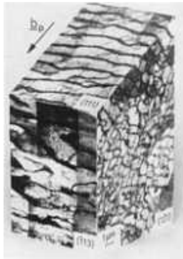
FIG. 17 THREE-DIMENSIONAL IMAGE OF THE DISLOCATION ARRANGEMENT OF MONOCRYSTALLINE COPPER IN CYCLIC SATURATION AT \gamma_{AP} = 1.45 \times 10^{-2} . SOURCE: REF 43
