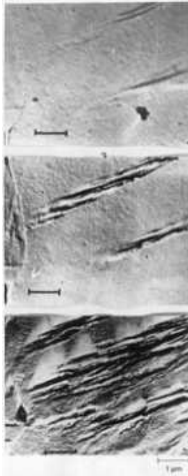
FIG. 2 EVOLUTION OF FATIGUE SLIP BANDS DURING CYCLING OF COPPER. (A) N = 5 \times 10^3 (B) N = 10^4 (C) N = 10^5 CYCLES. PUSH-PULL SYMMETRICAL LOADING ( R = -1 ) WITH LOW STRESS AMPLITUDES. NUMBER OF CYCLES TO FRACTURE, N_F = 1.2 \times 10^6 CYCLES
