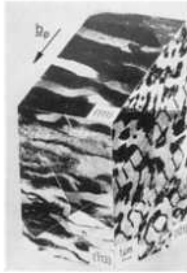
FIG. 14 THREE-DIMENSIONAL IMAGE OF THE DISLOCATION ARRANGEMENT OF CYCLIC SATURATION OF MONOCRYSTALLINE COPPER AT \gamma_{AP} = 1.5 \times 10^{-3} (REGION B). SOURCE: REF 46
