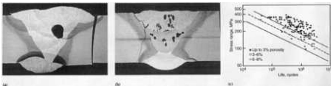
FIG. 11 EFFECT OF VOLUMETRIC DEFECTS ON FATIGUE. (A) SLAG INCLUSION IN BUTT WELD. CRACKING FROM WELD TOE. (B) POROSITY IN BUTT WELD. CRACKING FROM WELD TOE. (C) TRANSVERSE GROOVE WELDS CONTAINING POROSITY
