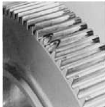
FIG. 5 MISALIGNED GEAR HAS TOOTH BREAKAGE AT ENDS OF TEETH.
