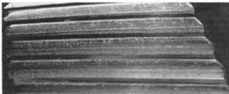
FIG. 10 HELICAL GEAR WITH SERIOUS LEDGE WEAR DUE TO MICRO- AND MACROPITTING
