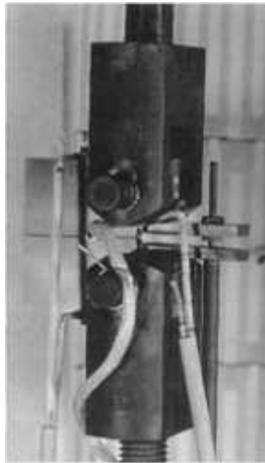
FIG. 10 TYPICAL INSTALLED SPECIMEN READY FOR CREEP CRACK GROWTH TESTING
