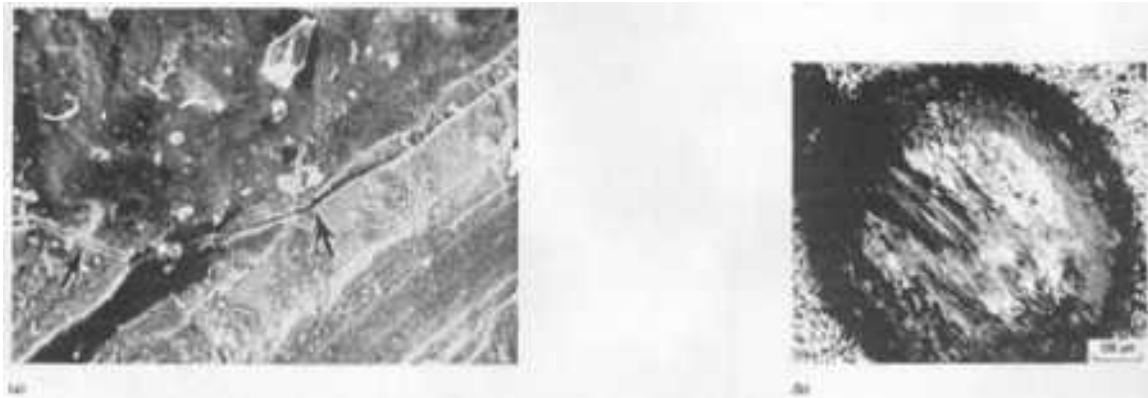
FIG. 2 FRETTING WEAR SCARS. (A) ON STEEL (ARROWS INDICATE FATIGUE CRACK). COURTESY OF R.B. WATERHOUSE, UNIVERSITY OF NOTTINGHAM. (B) ON HIGH-PURITY NICKEL. COURTESY OF R.C. BILL, NASA LEWIS RESEARCH CENTER
