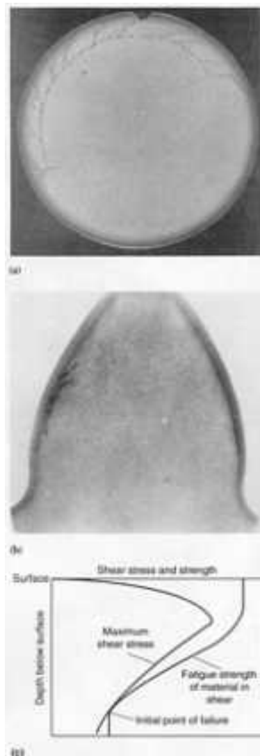
FIG. 7 MICROGRAPHS SHOWING ETCHED CROSS-SECTIONS OF (A) A CARBURIZED CYLINDRICAL TEST SPECIMEN (1.9 \times ) AND (B) A CARBURIZED GEAR TOOTH IN WHICH SUBCASE FATIGUE CRACKS INITIATED AND PROPAGATED DURING TESTING. SUBCASE FATIGUE, CALLED CASE CRUSHING BY PEDERSON AND RICE, SHOWS THE EARLY STAGES OF FATIGUE CRACKING IN THE LOWER CARBON PORTION OF THE CARBURIZED CASE. (C) THE DIAGRAM INDICATES HOW THE STRESS AND STRENGTH GRADIENTS COMBINE TO CAUSE THE WEAKEST CONDITION AT THE SUBCASE LOCATION WHERE FATIGUE CRACKING BEGINS. SOURCE: REF 26, 31, AND 33
