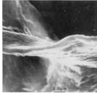
FIG. 10 PLASTIC CASTING OF FATIGUE CRACK IN 2024-T3. NOTE THE STRIATIONS, WAVY CRACK FRONT, AND ROUNDED CRACK TIP. SOURCE: REF 13
