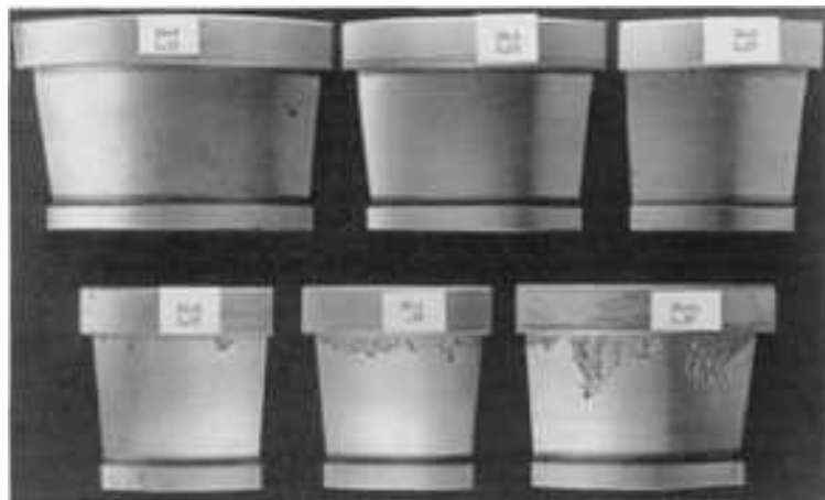
FIG. 5 FRACTOGRAPH SHOWING VARIOUS ADVANCED STAGES OF GEOMETRIC STRESS CONCENTRATION WITH MACROPITTING (SPALLING) FATIGUE OF BEARING RACEWAYS. RELATIVE LIFE NUMBERS ARE INDICATED TO SHOW THAT PROPAGATION IS NOT RELATED TO LIFE.
