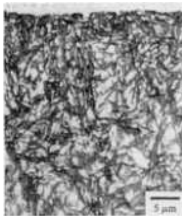
FIG. 1 TYPICAL NEAR-SURFACE CASE MICROSTRUCTURE OF DIRECT-QUENCHED CARBURIZED STEEL. MARTENSITE PLATES ETCH DARK AND RETAINED AUSTENITE APPEARS WHITE. GAS-CARBURIZED AISI 8719 STEEL (1.06% MN, 0.52% CR, 0.5% NI, 0.17% MO). LIGHT MICROGRAPH, NITAL ETCH
