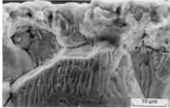
FIG. 16 SURFACE OXIDES ON A FRACTURE SURFACE FROM A SPECIMEN OF THE STEEL IDENTIFIED IN FIG. 15. SOURCE: REF 51
