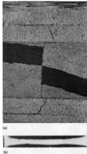
FIG. 4 DELAMINATION IN [0^\circ/\pm 45^\circ/90^\circ] GRAPHITE-EPOXY SUBJECTED TO STATIC LOADING. (A) MICROGRAPH OF A FREE EDGE. 35\times . (B) AN X-RAY OF THE WIDTH. 0.2\times
